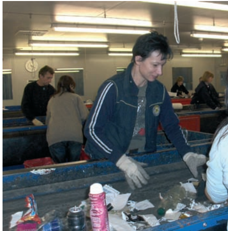
A lot of hand sorting is necessary at the Materials Recovery Facility.
