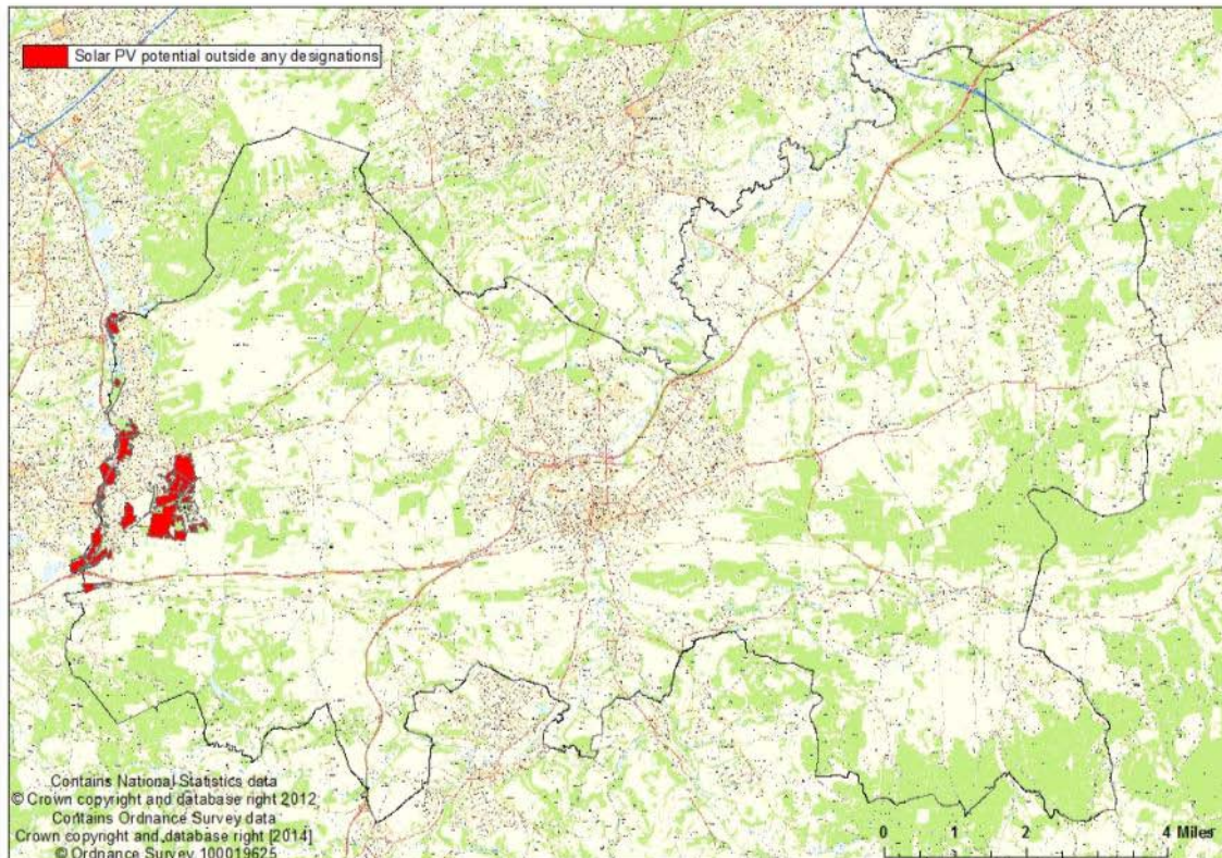
Figure 53: Potential for solar PV farms in Guildford Borough outside exclusion zones, AONB, SSSI, AGLV and green belt
