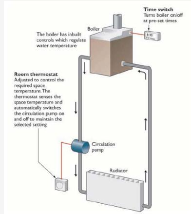
The boiler has inbuilt controls which regulate water temperature.
