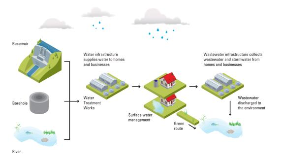
A broad overview of the water cycle and the role of wastewater infrastructure within the cycle is illustrated in Figure 3-1. Wastewater is generally produced following the use of potable water in homes, businesses, industrial processes and in certain areas can include surface water runoff (where sewerage networks are combined foul and surface water).
