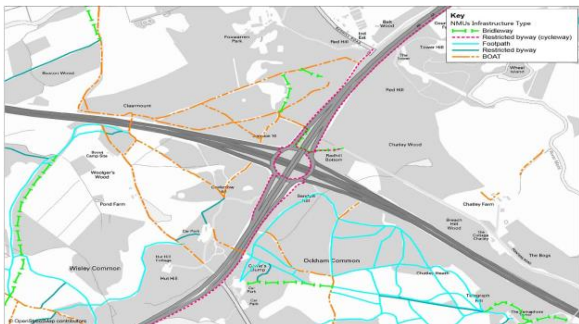
Figure 2-2 M25 Non-motorised users – current arrangements
