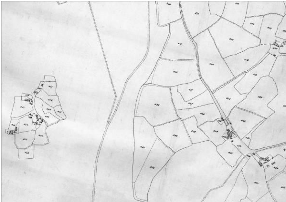
Figure 2. Example of a Tithe Map (1846). Drawn at a scale of 5 chains to 1" (20" to 1 mile). The detail in this figure shows the same area of the parish of Thursley as Figure 1. The quality of the tithe maps produced varies enormously; some were original surveys, others little more than topographical sketches or copies of slightly earlier maps. Some made elaborate use of colour to distinguish different properties, tithe free areas or land use, (see Figure 3); while others, like the one shown above, gave no such detail meaning the transcription of the associated apportionments was vital to their usefulness as a historical resource for the AWI revision.
