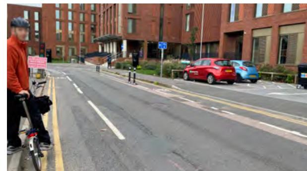
Figure 63. Existing modal filter on Walnut Tree Close allows northbound through traffic and restricts southbound through traffic. Cyclists are permitted bi-directionally. Proposal to restrict all through traffic and allow access only.
