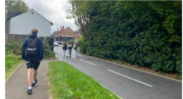
Figure 137. Uncontrolled crossing with footway missing on western side of The Street.
