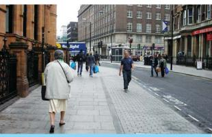
Raised Loading/Parking Pad Reallocates carriageway space to the footway, providing a wider, more comfortable pedestrian environment. The pads may be used for servicing or parking as needed, but allow a more flexible use of space to better accommodate pedestrians and narrow the carriageway.
