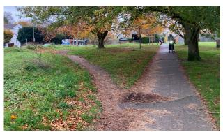
Figure 129. Shalford Park shared use path requires widening and resurfacing, as in many locations tree roots have damaged the surface. Existing desire lines to Pilgrims Way bus stop to be formalised.
